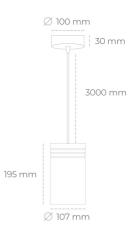
COB Light colour 2700 [K] | CRI Led chip flux 4311 [lm] Luminous flux 3879 [lm] System power 31 [W] Luminaire Efficiency 125 [lm/W] Beam angle 23° Controller ON/OFF MacAdam 3 SDCM
