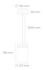
COB 4000 [K] HI EFFICIENT Light colour CRI 90 Led chip flux 3793 [lm] Luminous flux 3413 [lm] System power 23 [W] Luminaire Efficiency 148 [lm/W] Beam angle 60° Controller ON/OFF MacAdam 3 SDCM
