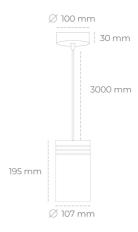
COB 4000 [K] HI EFFICIENT Light colour CRI 90 Led chip flux 2260 [lm] Luminous flux 2034 [lm] System power 14 [W] Luminaire Efficiency 145 [lm/W] Beam angle 23° Controller ON/OFF MacAdam 3 SDCM
