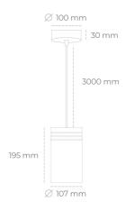
COB 3500 [K] HI EFFICIENT Light colour CRI 90 Led chip flux 3341 [lm] Luminous flux 3006 [lm] System power 21 [W] Luminaire Efficiency 143 [lm/W] Beam angle 60° Controller ON/OFF MacAdam 3 SDCM
