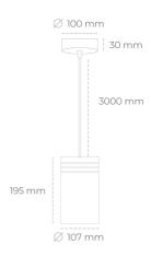
COB 3000 [K] HI EFFICIENT Light colour CRI 90 Led chip flux 3184 [lm] Luminous flux 2865 [lm] System power 19 [W] Luminaire Efficiency 151 [lm/W] Beam angle 38° Controller ON/OFF MacAdam 3 SDCM
