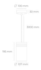
COB 3000 [K] HI EFFICIENT Light colour CRI 90 Led chip flux 2256 [lm] Luminous flux 2030 [lm] System power 14 [W] Luminaire Efficiency 145 [lm/W] Beam angle 15° Controller ON/OFF MacAdam 3 SDCM
