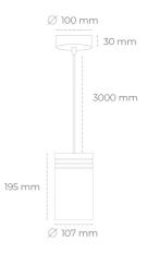
COB Light colour 3000 [K] | CRI 2997 [lm] Led chip flux Luminous flux 2697 [lm] System power 25 [W] Luminaire Efficiency 108 [lm/W] Beam angle 60° Controller ON/OFF MacAdam 3 SDCM
