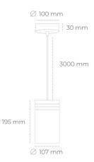
COB Light colour 3000 [K] | CRI Led chip flux 2536 [lm] Luminous flux 2282 [lm] System power 21 [W] Luminaire Efficiency 109 [lm/W] Beam angle 60° Controller ON/OFF MacAdam 3 SDCM
