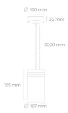
COB Light colour 2700 [K] | CRI Led chip flux 2222 [lm] Luminous flux 1999 [lm] System power 19 [W] Luminaire Efficiency 105 [lm/W] Beam angle 23° Controller ON/OFF MacAdam 3 SDCM
