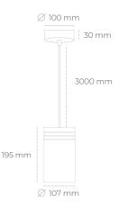
COB Light colour 4000 [K] | CRI Led chip flux 2839 [lm] Luminous flux 2555 [lm] System power 19 [W] Luminaire Efficiency 134 [lm/W] Beam angle 45° Controller ON/OFF MacAdam 3 SDCM
