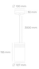
COB Light colour 4000 [K] | CRI Led chip flux 4542 [lm] Luminous flux 4087 [lm] System power 31 [W] Luminaire Efficiency 132 [lm/W] Beam angle 38° Controller ON/OFF MacAdam 3 SDCM
