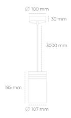
COB Light colour 4000 [K] | CRI Led chip flux 2839 [lm] Luminous flux 2555 [lm] System power 19 [W] Luminaire Efficiency 134 [lm/W] Beam angle 38° Controller ON/OFF MacAdam 3 SDCM
