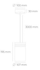
COB Light colour 3500 [K] | CRI 3896 [lm] Led chip flux Luminous flux 3506 [lm] System power 27 [W] Luminaire Efficiency 130 [lm/W] Beam angle 60° Controller ON/OFF MacAdam 3 SDCM
