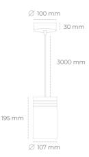
COB Light colour 3500 [K] | CRI Led chip flux 2783 [lm] Luminous flux 2504 [lm] System power 19 [W] Luminaire Efficiency 132 [lm/W] Beam angle 38° Controller ON/OFF MacAdam 3 SDCM
