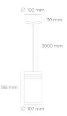
COB Light colour 3500 [K] | CRI 1948 [lm] Led chip flux Luminous flux 1753 [lm] System power 14 [W] Luminaire Efficiency 125 [lm/W] Beam angle 23° Controller ON/OFF MacAdam 3 SDCM
