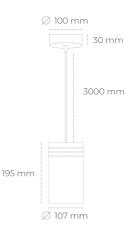
COB Light colour 3500 [K] | CRI Led chip flux 3618 [lm] Luminous flux 3256 [lm] System power 25 [W] Luminaire Efficiency 130 [lm/W] Beam angle 15° Controller ON/OFF MacAdam 3 SDCM
