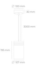
COB Light colour 3500 [K] | CRI Led chip flux 1391 [lm] Luminous flux 1251 [lm] System power 10 [W] Luminaire Efficiency 125 [lm/W] Beam angle 15° Controller ON/OFF MacAdam 3 SDCM
