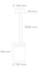
COB Light colour 3000 [K] | CRI 2994 [lm] Led chip flux Luminous flux 2694 [lm] System power 21 [W] Luminaire Efficiency 128 [lm/W] Beam angle 15° Controller ON/OFF MacAdam 3 SDCM
