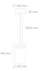
COB Light colour 3000 [K] | CRI Led chip flux 2722 [lm] Luminous flux 2449 [lm] System power 19 [W] Luminaire Efficiency 129 [lm/W] Beam angle 15° Controller ON/OFF MacAdam 3 SDCM
