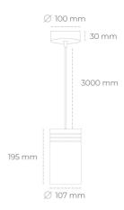
COB 4200 [K] MEAT WHITE Light colour CRI 90 Led chip flux 1976 [lm] Luminous flux 1778 [lm] System power 19 [W] Luminaire Efficiency 94 [Im/W] Beam angle 38° Controller ON/OFF MacAdam 3 SDCM
