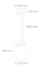
COB 3000 [K] HI EFFICIENT Light colour CRI 90 Led chip flux 1623 [lm] Luminous flux 1460 [lm] System power 10 [W] Luminaire Efficiency 146 [lm/W] Beam angle 45° Controller ON/OFF MacAdam 3 SDCM
