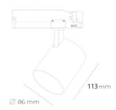
COB 3000 [K] CRI97 Light colour CRI Led chip flux 2601 [lm] Luminous flux 2340 [lm] System power 23 [W] Luminaire Efficiency 102 [lm/W] Beam angle 23° Controller ON/OFF
