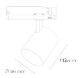
COB Light colour 3500 [K] | CRI Led chip flux 2783 [lm] Luminous flux 2504 [lm] System power 19 [W] Luminaire Efficiency 132 [lm/W] Beam angle 45° Controller ON/OFF MacAdam 3 SDCM
