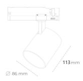
COB 3500 [K] HI EFFICIENT Light colour CRI 90 Led chip flux 3624 [lm] Luminous flux 3261 [lm] System power 23 [W] Luminaire Efficiency 142 [lm/W] Beam angle 38° Controller ON/OFF MacAdam 3 SDCM
