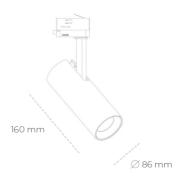
COB 3500 [K] HI EFFICIENT Light colour CRI 90 Led chip flux 3054 [lm] Luminous flux 2748 [lm] System power 19 [W] Luminaire Efficiency 145 [lm/W] Beam angle 60° Controller ON/OFF MacAdam 3 SDCM
