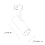
COB 4000 [K] HI EFFICIENT Light colour CRI 90 Led chip flux 2260 [lm] Luminous flux 2034 [lm] System power 14 [W] Luminaire Efficiency 145 [lm/W] Beam angle 60° Controller ON/OFF MacAdam
