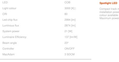
Compact track mounted LED spotlight. Aluminium housing. Ceiling base installation possible. Available in white, black and grey. Any RAL palette colour available on enquiry. Reflector beams available: 15°, 24°, 38° and 60°. Maximum power is 31W
