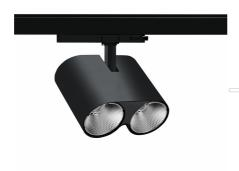
COB 4000 [K] HI EFFICIENT Light colour CRI Led chip flux 3492 [lm] Luminous flux 3352 [lm] System power 21 [W] Luminaire Efficiency 160 [lm/W] Beam angle 38° Controller ON/OFF MacAdam 3 SDCM
