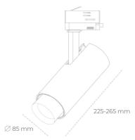
COB 3500 [K] PREMIUM WHITE Light colour CRI 90 Led chip flux 3513 [lm] Luminous flux 2107 [lm] System power 23 [W] Luminaire Efficiency 92 [lm/W] Beam angle 36° Controller ON/OFF MacAdam 3 SDCM
