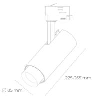
COB 4000 [K] HI EFFICIENT Light colour CRI 90 Led chip flux 3492 [lm] Luminous flux 2095 [lm] System power 21 [W] Luminaire Efficiency 100 [lm/W] Beam angle 36° Controller ON/OFF MacAdam 3 SDCM
