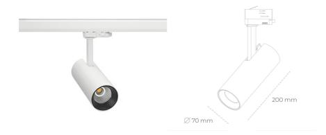
COB 2500 [K] BREAD Light colour CRI 2340 [lm] Led chip flux Luminous flux 1872 [lm] System power 19 [W] Luminaire Efficiency 99 [lm/W] Beam angle 24° Controller ON/OFF
