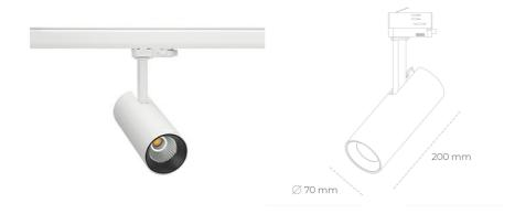
COB 2500 [K] BREAD Light colour CRI 1674 [lm] Led chip flux Luminous flux 1339 [lm] System power 14 [W] Luminaire Efficiency 96 [lm/W] Beam angle 15° Controller ON/OFF MacAdam 3 SDCM
