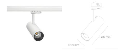
COB 3000 [K] CRI97 Light colour CRI Led chip flux 1575 [lm] Luminous flux 1260 [lm] System power 14 [W] Luminaire Efficiency 90 [lm/W] Beam angle 15° Controller ON/OFF MacAdam 3 SDCM
