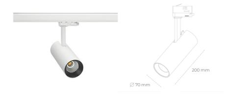
COB 5700 [K] SPECIAL Light colour CRI Led chip flux 1820 [lm] Luminous flux 1456 [lm] System power 14 [W] Luminaire Efficiency 104 [lm/W] Beam angle 38° Controller ON/OFF
