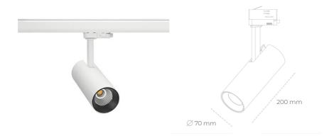
COB 4200 [K] MEAT WHITE Light colour CRI 90 Led chip flux Luminous flux 818 [lm] System power 10 [W] Luminaire Efficiency 82 [lm/W] Beam angle 38° Controller ON/OFF MacAdam 3 SDCM
