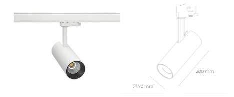
COB 4200 [K] MEAT WHITE Light colour CRI 90 Led chip flux 2159 [lm] Luminous flux 1727 [lm] System power 21 [W] Luminaire Efficiency 82 [lm/W] Beam angle 24° Controller ON/OFF MacAdam 3 SDCM
