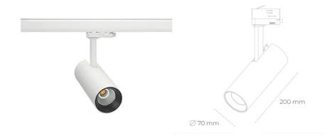
COB 4200 [K] MEAT WHITE Light colour CRI 90 Led chip flux 1412 [lm] Luminous flux 1129 [lm] System power 14 [W] Luminaire Efficiency 81 [lm/W] Beam angle 15° Controller ON/OFF MacAdam 3 SDCM
