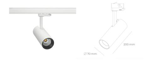
COB 3000 [K] HI EFFICIENT Light colour CRI 90 Led chip flux 3487 [lm] Luminous flux 2789 [lm] System power 21 [W] Luminaire Efficiency 133 [lm/W] Beam angle 60° Controller ON/OFF MacAdam 3 SDCM
