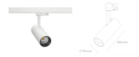
COB 3000 [K] HI EFFICIENT Light colour CRI 90 Led chip flux 3487 [lm] Luminous flux 2789 [lm] System power 21 [W] Luminaire Efficiency 133 [lm/W] Beam angle 38° Controller ON/OFF MacAdam 3 SDCM
