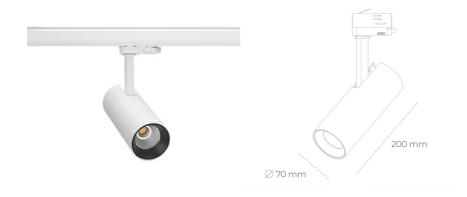
COB 3000 [K] HI EFFICIENT Light colour CRI 90 Led chip flux 3184 [lm] Luminous flux 2547 [lm] System power 19 [W] Luminaire Efficiency 134 [lm/W] Beam angle 38° Controller ON/OFF MacAdam 3 SDCM
