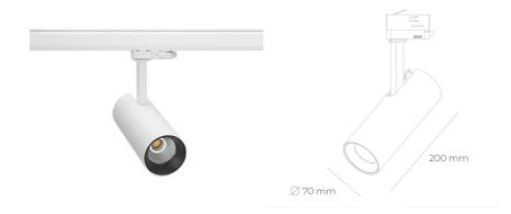
COB 3000 [K] HI EFFICIENT Light colour CRI 90 Led chip flux 2256 [lm] Luminous flux 1804 [lm] System power 14 [W] Luminaire Efficiency 129 [lm/W] Beam angle 15° Controller ON/OFF MacAdam 3 SDCM
