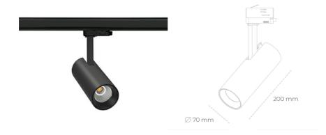
COB 2500 [K] BREAD Light colour CRI 2574 [lm] Led chip flux Luminous flux 2059 [lm] System power 21 [W] Luminaire Efficiency 98 [lm/W] Beam angle 60° Controller ON/OFF MacAdam 3 SDCM
