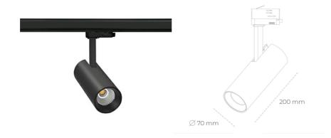
COB 3000 [K] PREMIUM COLOR Light colour CRI 90 Led chip flux 1145 [lm] Luminous flux 916 [lm] System power 11 [W] Luminaire Efficiency 83 [lm/W] Beam angle 15° Controller ON/OFF MacAdam
