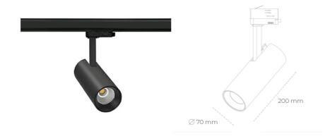
COB 5700 [K] SPECIAL Light colour CRI 2788 [lm] Led chip flux Luminous flux 2230 [lm] System power 21 [W] Luminaire Efficiency 106 [lm/W] Beam angle 60° Controller ON/OFF MacAdam 3 SDCM
