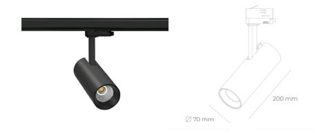
COB 5700 [K] SPECIAL Light colour CRI 2788 [lm] Led chip flux Luminous flux 2230 [lm] System power 21 [W] Luminaire Efficiency 106 [lm/W] Beam angle 24° Controller ON/OFF MacAdam 3 SDCM
