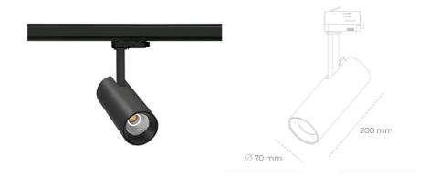
COB 4200 [K] MEAT WHITE Light colour CRI 90 Led chip flux Luminous flux 818 [lm] System power 10 [W] Luminaire Efficiency 82 [lm/W] Beam angle 60° Controller ON/OFF MacAdam 3 SDCM
