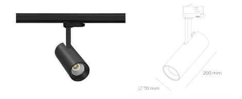
COB 4200 [K] MEAT WHITE Light colour CRI 90 Led chip flux Luminous flux 818 [lm] System power 10 [W] Luminaire Efficiency 82 [lm/W] Beam angle 38° Controller ON/OFF MacAdam 3 SDCM
