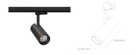
COB 4000 [K] HI EFFICIENT Light colour CRI 90 Led chip flux 3189 [lm] Luminous flux 2551 [lm] System power 19 [W] Luminaire Efficiency 134 [lm/W] Beam angle 38° Controller ON/OFF MacAdam 3 SDCM
