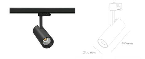
COB 4000 [K] HI EFFICIENT Light colour CRI 90 Led chip flux 2260 [lm] Luminous flux 1808 [lm] System power 14 [W] Luminaire Efficiency 129 [lm/W] Beam angle 38° Controller ON/OFF MacAdam 3 SDCM
