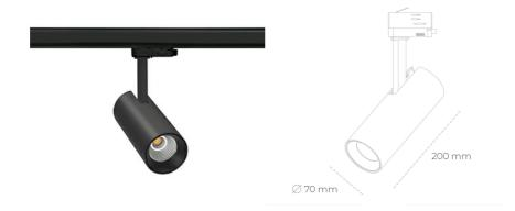
COB 4000 [K] HI EFFICIENT Light colour CRI 90 Led chip flux 1625 [lm] Luminous flux 1300 [lm] System power 10 [W] Luminaire Efficiency 130 [lm/W] Beam angle 38° Controller ON/OFF MacAdam 3 SDCM
